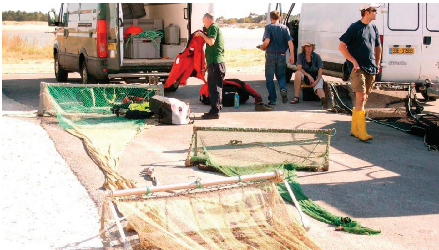
Intercalibration on a European scale helps to make the data comparable. After comparing several techniques, the beam trawl was chosen for sampling fish in estuaries.
